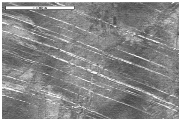
Fig. 21. SEM-ECC picture for 30 GPa shocked [221] Cu samples: front surface of the sample perpendicular to the shock propagation direction [87].
